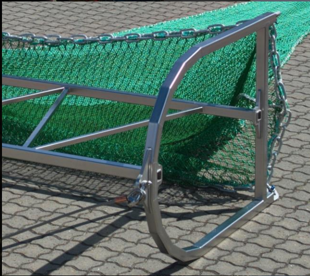
(b) Small Agassiz Trawl 135 cm x 70 cm (width x height) mesh size 10 mm
