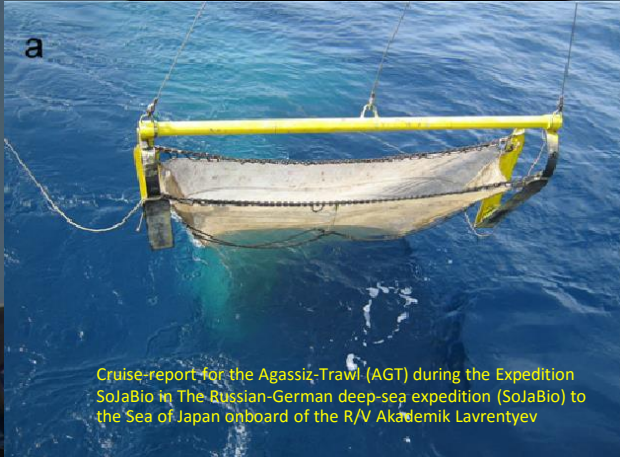
(a) Typical Agassiz Trawl 350 cm x 70 cm (width x height) mesh size 10 mm
