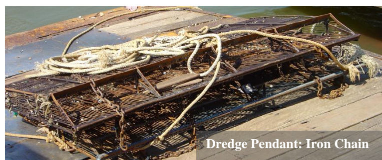
Figure 20 Iron dredge construction
