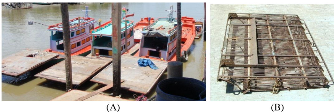
Figure 26 (A) Medium scale fishing boat, length over all (LOA) 12-14 m, operate without deck machinery (B) Medium scale iron dredge, entrance length is 2.0-2.4 m
