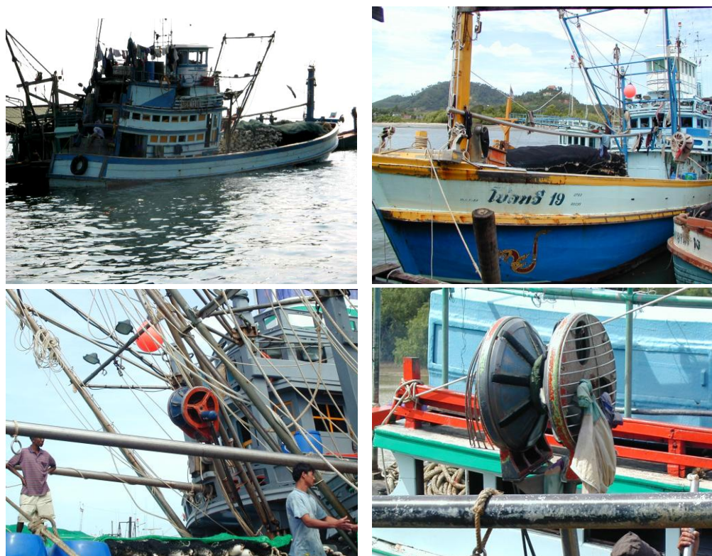
Fig. 16. Purse seiner of surrounding net with a purse line (mesh size 25.0-29.9 mm)
