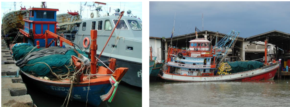
Fig. 13. Purse seiner of surrounding net with a purse line (mesh size less than 10 mm) Left: Thai model; Right: Malaysian model Photo by SEAFDEC (2004) and A. Munprasit (2009)
