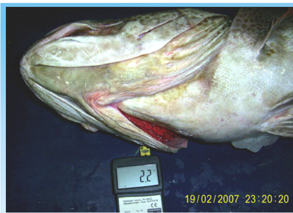
Figure 11. Temperature of fish 4 and half hours in slush chilled seawater down to 2.2°C
