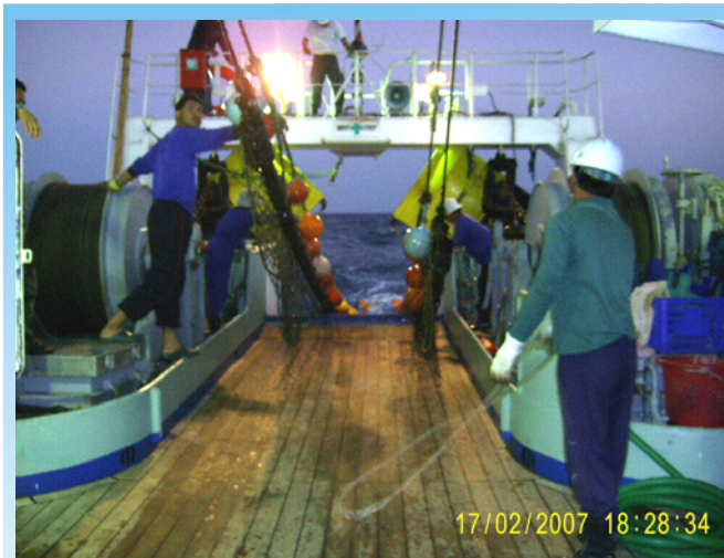
Figure 2. Preparing the M.V. SEAFDEC 2 for onboard handling with the use of a deck hose to cool down the working area
